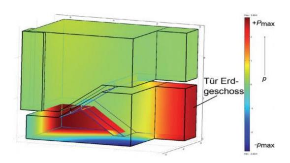
Sound pressure distribution computed at the resonance frequency of 38.5 Hz in a staircase. Due to the sound of a closing door, this resonance is particularly strong because the door is located exactly at the sound pressure maximum (red:
