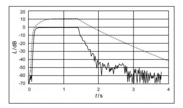
Level slope without (continuous line) and with (dashed line) the optimized resonator. Credit: PTB
