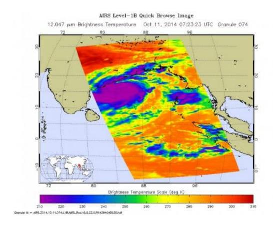
The AIRS instrument aboard Aqua captured infrared data on the storm that showed cloud top temperatures had dropped, indicating stronger uplift and stronger thunderstorms. Credit: NASA JPL, Ed Olsen
