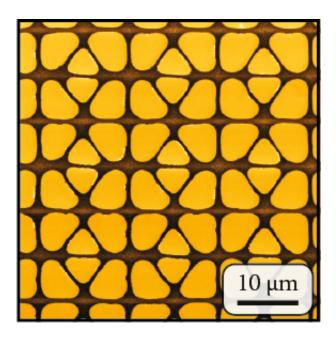
Nanostructures of virtually any possible shape can now be made using a combination of techniques developed by the MESA+ Institute for Nanotechnology of the University of Twente. Especially the unique properties of so-called perovskites can be exploited further: their crystal structure is not influenced by the process. The UT scientists present their findings in the journal *Advanced Functional Materials*.
