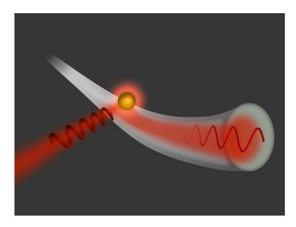
Light hits a gold particle, which then emits light into a glass fibre - into only one direction.
