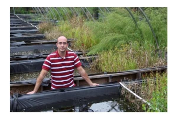
Nanotechnology researcher Lee Ferguson stands amid a collection of simulated wetlands called mescosms at Duke University. Each wetland-in-a-box is used to run the experiment under varying conditions.
