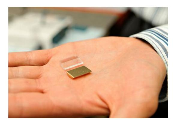
The gold nanonparticules on the surface of this receiving tab modify the colour of light detected by the instrument. The captured colour perfectly reflects the exact concentration of the medication in the blood sample. Credit: University of Montreal
