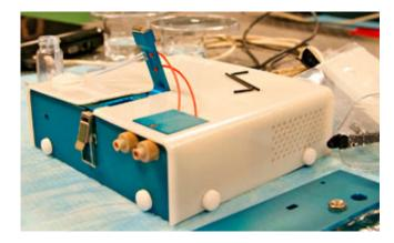
As preicse yet 10 times less expensive than current hospital equipment, this little device contains an optical system that enables it to rapidly identify the dose of methotrexate that a cancer requires, minimising the drugs undesirable side effects. Credit: University of Montreal
