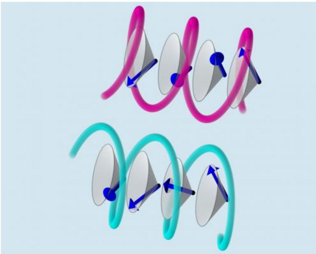
Figure 1: Multiferroics have a screw spin structure (arrows) with clockwise (lower) and anticlockwise (upper) orientations that can control the propagation of light at terahertz and gigahertz frequencies. Credit: Youtarou Takahashi, RIKEN Center for Emergent Matter Science
