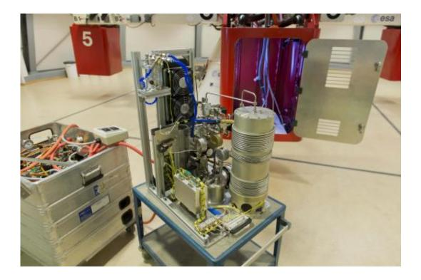
A furnace for the solidification of titanium aluminide (TiAl) alloy ready to be placed into its Large Diameter Centrifuge gondola. The furnace chamber at the cylinder's core is surrounded by ceramic heatshields and buffered by inert argon gas, with telemetry systems and external water-cooling pipes seen wrapped around the cylinder. Credit: ESA–A. Le Floc'h
