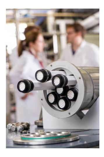
Preliminary concentration: Ceramic hollow fiber membranes are used to remove proteins from milk. Credit: A. Eckert / TUM
