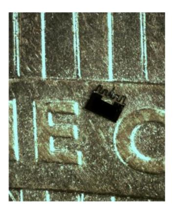
This image shows a "microforce-sensing mobile microrobot" juxtaposed against a U.S. penny. The device is being developed at Purdue University. Credit: Purdue University
