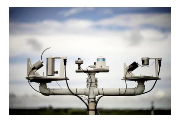
The Dual Multifilter Rotating Shadowband Radiometer takes spectral measurements of direct, diffuse, and total horizontal solar irradiances. Instruments such as these, located at the Southern Great Plains site in Oklahoma help scientists understand the amount and type of light that hits Earth's surface. Credit: ARM Climate Research Facility.
