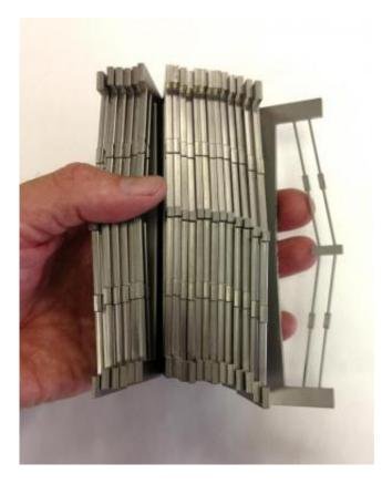
This image shows a stack of structural components called bistable springs. Credit: NASA/JPL-Caltech
