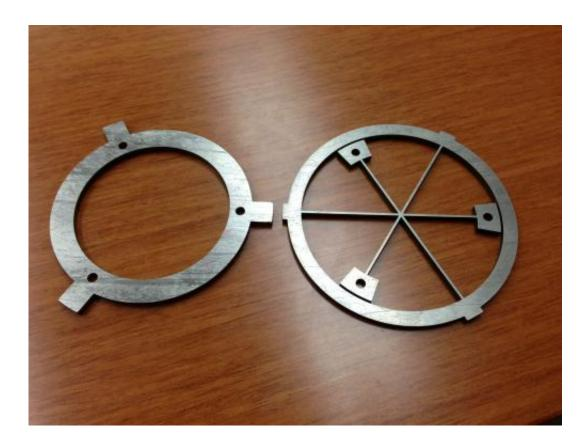
This image shows components of a mirror structure that can be rotated very precisely by flexing parts made of a material scientists call "bulk metallic glass." Credit: NASA/JPL-Caltech
