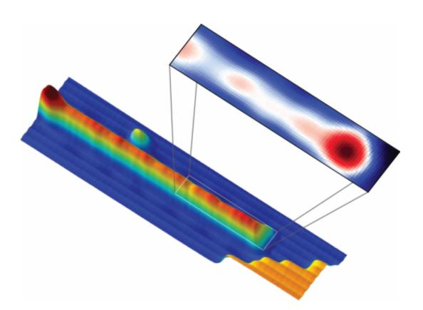
Princeton University scientists used scanning-tunneling microscope to show the atomic structure of an one-atom-wide iron wire on a lead surface. The zoomed-in portion of the image depicts the quantum probability of the wire containing an elusive particle called the Majorana fermion. Importantly, the image pinpoints the particle to the end of the wire, which is where it had been predicted to be over years of theoretical calculations. Credit: Yazdani Lab, Princeton University
