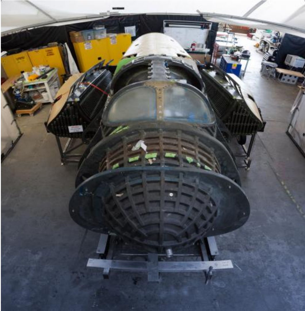
View of the Lynx cockpit, fuselage and strakes. Credit: XCOR Aerospace / Mike Masee
