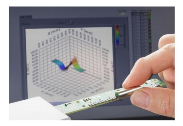
The line camera visualizes magnetic field values in real time. Credit: Max Etzold
