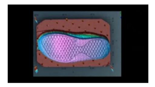
Researchers at the National Institute of Standards and Technology have demonstrated a laser-based imaging system that creates high-definition 3D maps of surfaces from as far away as 10.5 meters. The method may be useful in diverse fields, including precision machining and assembly, as well as in forensics.
