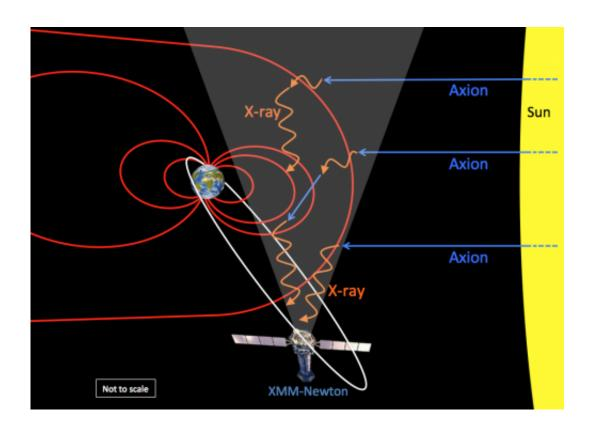
A sketch (not to scale) showing axions (blue) streaming out from the Sun, converting in the Earth's magnetic field (red) into X-rays (orange), which are then detected by the XMM-Newton observatory. (copyright University of Leicester
