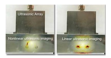
The next generation of aircraft could be thinner and lighter thanks to the development of a new imaging technique that could detect damage previously invisible to acoustic imaging systems.
