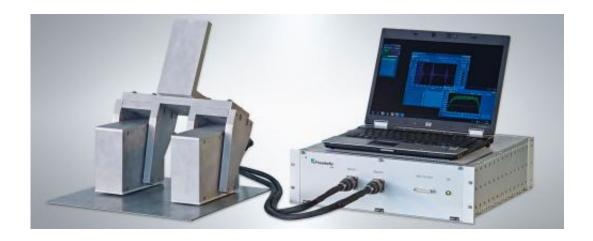
Hybrid micromagnetics/ultrasound inspection system. Credit: Uwe Bellhäuser, Fraunhofer IZFP
