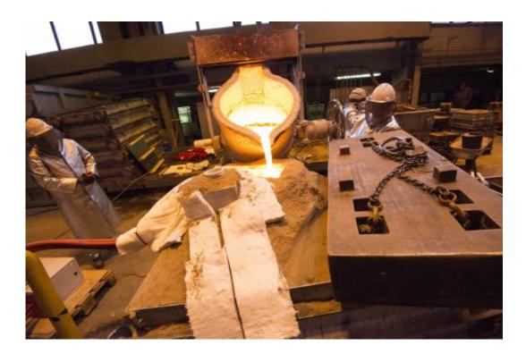
New technology almost halves the amount of metal that has to be melted in order to cast a propeller blade. This was tested for the first time on an industrial scale at Oshaug Metall in Molde. Credit: Oshaug Metall/Arnt Jørgen Sønslien
