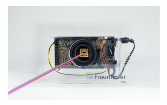
Emission spectrometers analyze materials on the basis of their emitted light spectrum. Novel sensors permit the development of even smaller, faster and more precise test instruments. Credit: Fraunhofer IMS
