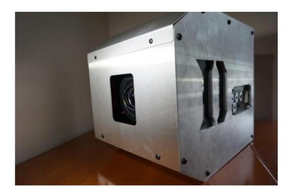
This unique instrument simultaneously photographs a 2 meter tall individual to 75 micron resolution. Credit: Daniel Marks
