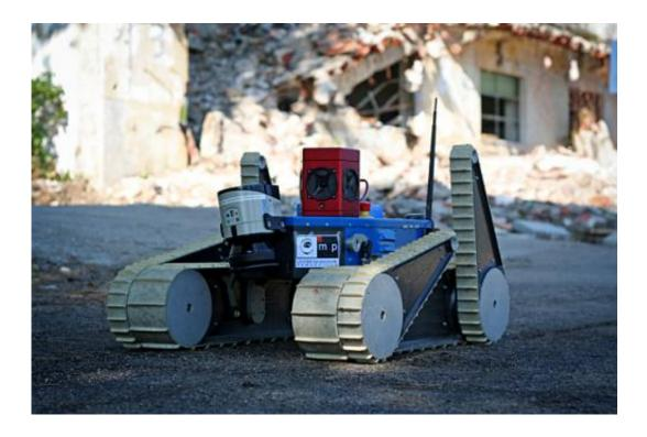
The robot that firefighters tested in Italy was found to be easier to use with the "free look control" method.
