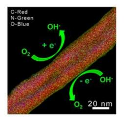
N-doped coaxial carbon nanocables with active sites effectively exposed at the surface for oxygen reduction and evolution reaction. (Image: Department of Chemical Engineering, Tsinghua University)
