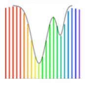
Molecular absorption profile superimposed on the modes of an optical frequency comb. Credit: NIST
