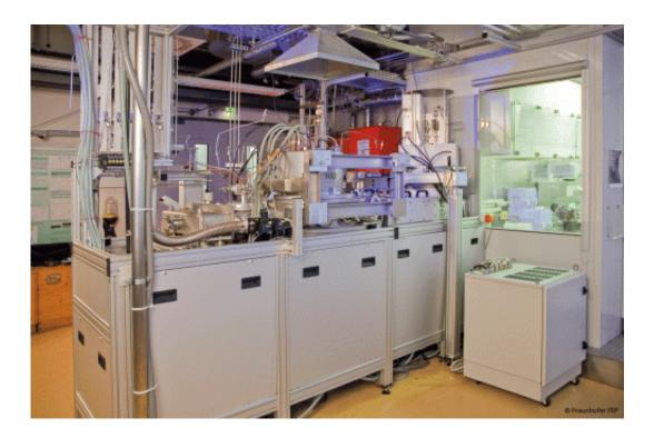
Fraunhofer researchers are using this lab coater to produce piezoelectric AlN layers for low power sensors in an economically feasible manner. Credit: Fraunhofer FEP
