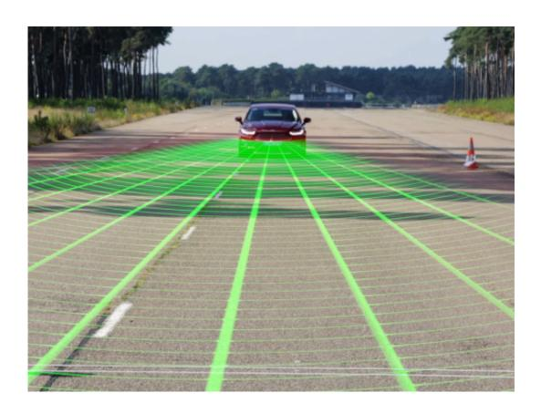
Pre-Collision Assist with Pedestrian Detection uses radar and camera technology to scan the roadway ahead and, if a collision risk with a vehicle or pedestrian is detected, provides a warning to the driver. If the
