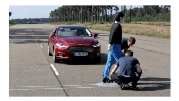
Ford Pre-Collision Assist with Pedestrian Detection Technology, available new technology from Ford is designed to reduce the severity of and, in some cases, even eliminate frontal collisions involving pedestrians. Debuting on the 2015 Ford Mondeo in Europe, the system provides a collision warning to the driver and, if the driver does not respond in time, can automatically apply the vehicle brakes.
