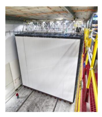
A man stands near the partially completed NOvA far detector in Ash River, Minnesota. The detector, constructed entirely of PVC, stands 50 feet tall and 50 feet wide. The completed detector is roughly 200 feet long. The NOvA team
