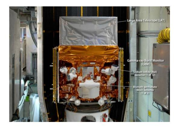
This image of NASA's Fermi Gamma-ray Space Telescope, shown here in May 2008 being readied for launch, highlights the spacecraft's instruments. The Gamma-ray Burst Monitor (GBM) is an array of 14 crystal detectors sensitive to short-lived gamma-ray blasts. Credit: NASA/Jim Grossmann
