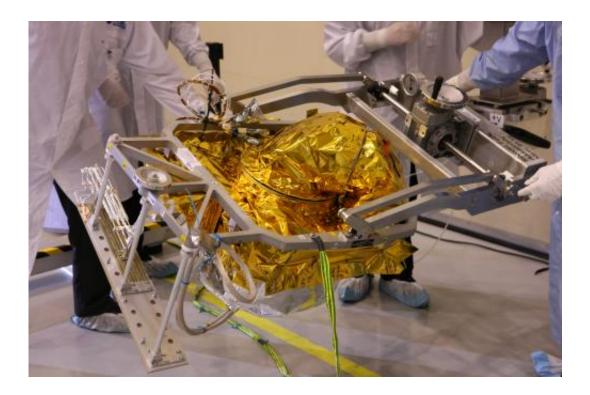
The Tesat Spacecom laser communication terminal is integrated on the Eutelsat-9B satellite in Airbus Defence and Space facilities in Toulouse, France. Credit: Airbus Defence and Space SAS
