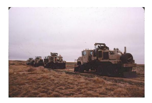
They used the vibroseis seismic reflection technique for this survey, whereby a series of trucks create a seismic signal by vibrating heavy plates laid on the ground through a series of known frequencies. Credit: Riff Raf
