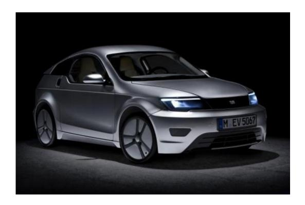
Visio.M: lightweight, highly efficient and safe, with timeless, modern and functional design. 15 kW are enough to reach a top speed of 120 km/h (75 mph). Credit: Florian Lehmann / TUM
