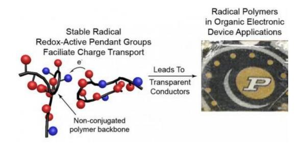
An emerging class of electrically conductive plastics are called "radical polymers." The graphic at left depicts the structure of a polymer. At right, transparent polymer overlays the Purdue logo. Credit: Purdue University
