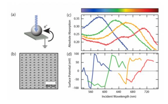
The newly discovered plasmoelectric effect. (a) Schematic representation of a metal nanosphere that becomes electrically charged when illuminated with light. (b) Electron microscope image of the metal nanocircuit made up from a matrix of ultra-small holes in a thin gold film. (c) Optical absorption spectra measured for metal nanocircuits with varying distances between the holes (175, 225, 250 and 300 nanometres). (d) Electrical potential of the nanocircuits in (c), as a
