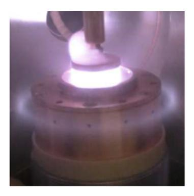
A laboratory test of a liquid-metal cathode. Credit: Photo courtesy of General Electric
