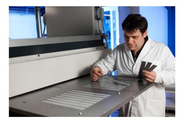
A scientist removing samples of electrical steel from the test facility at Fraunhofer IWS; this type of material is one of the main components of transformers. Credit: Fraunhofer IWS
