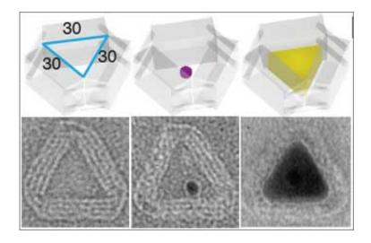
By creating molds from stiff DNA, researchers were able to cast gold "seeds" into complex metal nanoparticles. From left to right, this 3D polygonal particle was formed by designing a DNA mold, planting a gold seed, then chemically forcing the seed to expand until complete formation. Credit: Harvard's Wyss Institute
