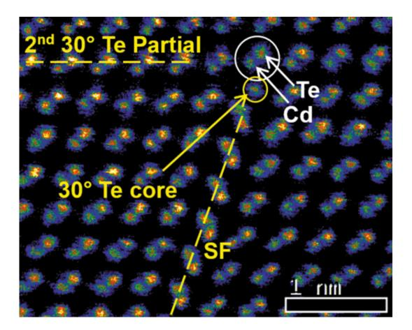
An image of an isolated  $30^{\circ}$  partial dislocation with Te core. Credit: Paulauskas et al
