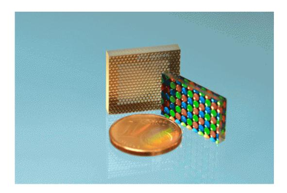
Micro-optical array projectors: Double-sided lens array with buried slide array (left) and lens array with buried color filters for LCD micro-imager (right). Credit: Fraunhofer IOF
