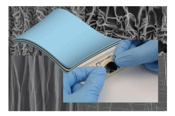
A diagram of the crumpled-graphene supercapacitor (upper left). The top and bottom layers are the polymer used as a substrate, the two dark layers are the crumpled graphene paper, and the middle layer, shown in white, is the hydrogel, used as an electrolyte. The inset photo shows the actual supercapacitor, demonstrating how it can be bent without affecting its electrical properties.
