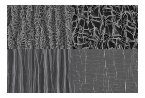
To form the crumpled graphene, a sheet of polymer material is stretched in both dimensions, then graphene paper is bonded to it. When the polymer is released in one direction, the graphene forms pleats, as shown in the bottom images, taken with a scanning electron microscope (SEM). Then, when released in the other direction, it forms a chaotic crumpled pattern (top images). The right pair of SEM images shows the material at higher magnification than the left-hand images.
