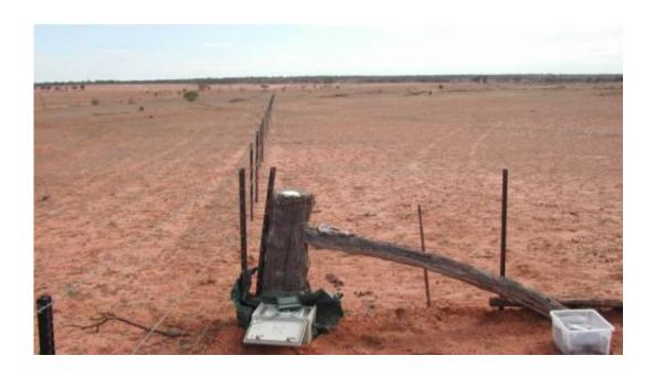
Seismic recorders placed around southeast Australia were used to record the data
