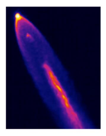
Thermal imagery of the Space X Falcon 9 first stage performing propulsive descent Sept. 21. Supersonic retropropulsion data obtained from this flight test is being analyzed by NASA to design future Mars landing systems. Credit: NASA
