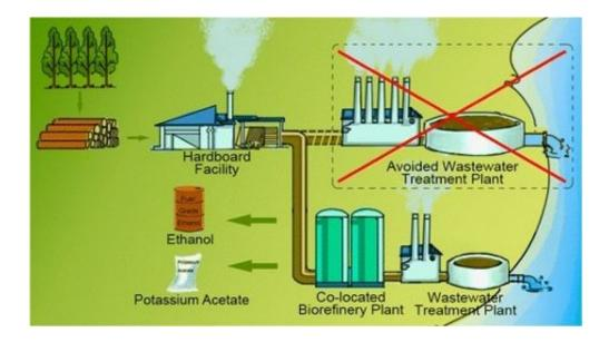
A co-located biorefinery and hardwood panel manufacturing plant. Reprinted with permission from ACS Sustainable Chemistry & Engineering. Copyright 2014. American Chemical Society.
