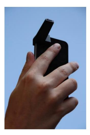
The iSPEX spectropolarimetric add-on is mounted in front of a smartphone camera, turning it into an optical device that measures aerosol properties. Measurements by thousands of participants in the iSPEX citizen science experiment match Aerosol Optical Thickness data from the ground-based AERONET station and the MODIS satellite. The iSPEX measurements add crucial information about aerosols that is not sampled by professional equipment.
