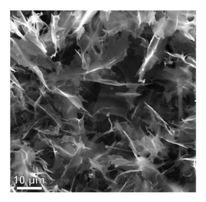
An electron microscope image shows flake-like nanoplatelets made of graphene quantum dots drawn from coal and graphene oxide sheets, modified with boron and nitrogen. The nanoplatelets feature enough edge to make them suitable as catalysts for applications like fuel cells. Courtesy of the Tour Group
