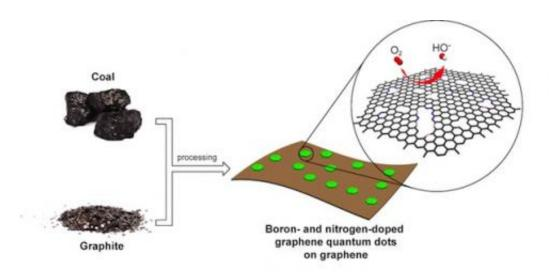
Rice University scientists combined graphene quantum dots, graphene oxide, nitrogen and boron into a catalyst capable of replacing platinum in fuel cells at a fraction of the cost. Illustration courtesy of the Tour Group
