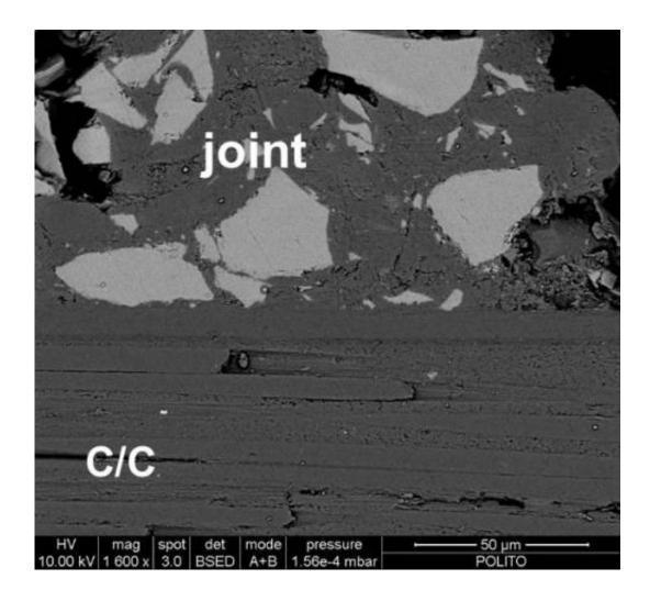
Scanning electron microscope image of silicon adhesive incorporating ceramic fillers, used to join carbon–carbon panels. The addition of the ceramic fillers helps to ensure its thermal and moisture expansion remains small enough for the kind of ultrastable structural performance required for future space missions. Credit: ESA/Thales Alenia Space
