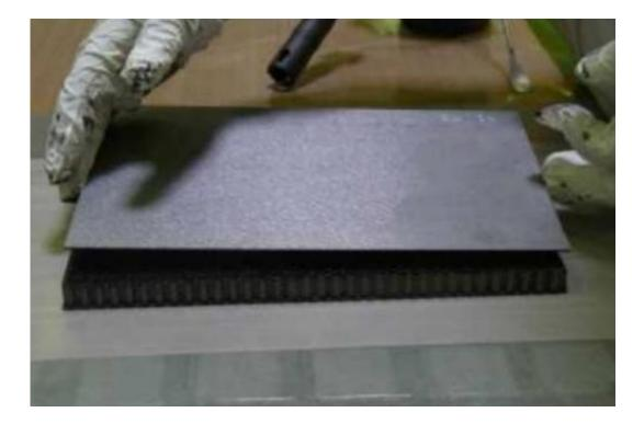
A carbon–carbon face being added to a carbon-carbon honeycomb, forming the top of a 'sandwich' panel. Carbon–carbon is formed from high-strength carbon fibres embedded in a graphite mix, resulting in a material that is lighter than aluminium while stronger than steel. Similar carbon composites have found uses in high-performance industries from aerospace to Formula One. Credit: ESA/Thales Alenia Space
