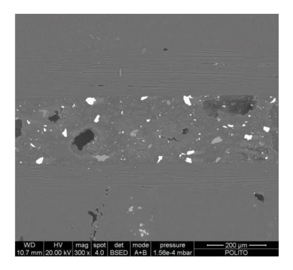
Microscope image of modified adhesive containing ceramic fillers used to join two carbon–carbon panels, intended to create ultrastable structures insensitive to temperature or moisture changes for future space missions. Credit: ESA/Thales Alenia Space
