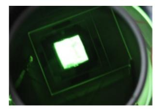
This is a plane-lighting homogeneity image of a planar light source device through a neutral density filter. Credit: N.Shimoi/Tohoku University
