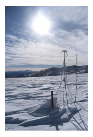
Some of the initial research involving GPS and snow-depth measurement took place at the Niwot Ridge field site, located in the foothills above Boulder, starting in 2009. Credit: Ethan Gutmann, NCAR.
