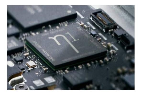
Eta Devices' chip (depicted here) can essentially "switch gears" to adjust voltage supply to power amplifiers in smartphones as needed, cutting power loss to improve battery life. Credit: Eta Devices
