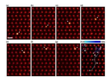
Selected frames from a sequence of scanning transmission electron microscope images showing the diffusion pathway of a Ce dopant (the bright atom highlighted with a white arrow) as it moves inside a bulk AlN crystal. The final frame overlays the Ce pathway on the Z-contrast image obtained by averaging each frame. Credit: Oak Ridge National Laboratory
